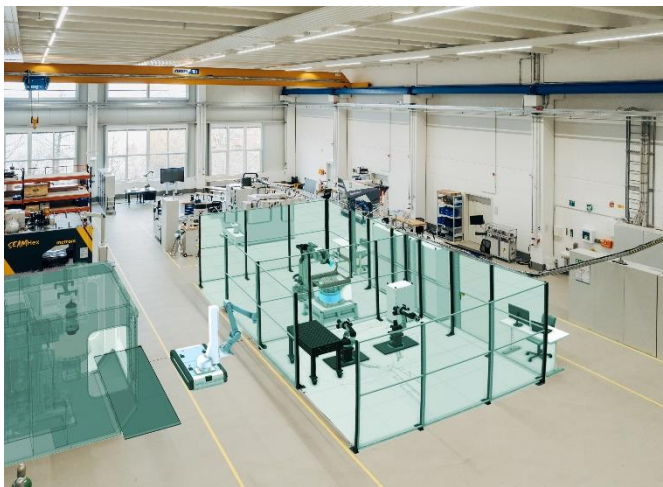
Fig. 1 Matrix architecture at the IWU location in Dresden (Pforzheimer Straße): flexibly designed production cells. The test field exists not only physically; a digital twin allows for variant investigations and optimizations (shown here in the rendering) © Fraunhofer IWU
