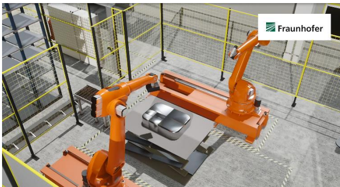
Fig. 2 SWAP enables the production of large components using small standard machines and a mobile machine for finishing © Fraunhofer
