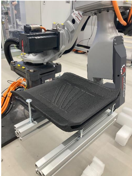
Fig. 3 Interconnecting standard machines and manufacturing components flexibly: production of a seat shell as one out of many possible applications
